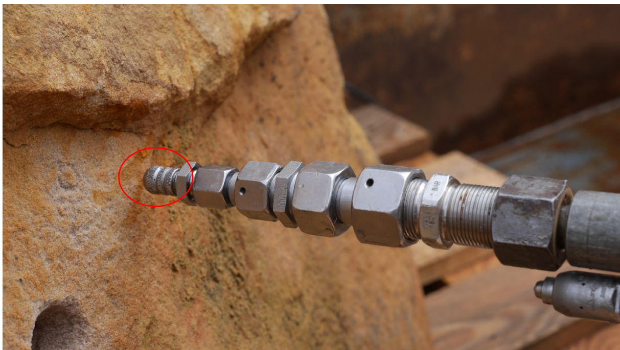
figure 4: static type RJD nozzle (first component on top, marked in red) during experiments with multiple adapters
