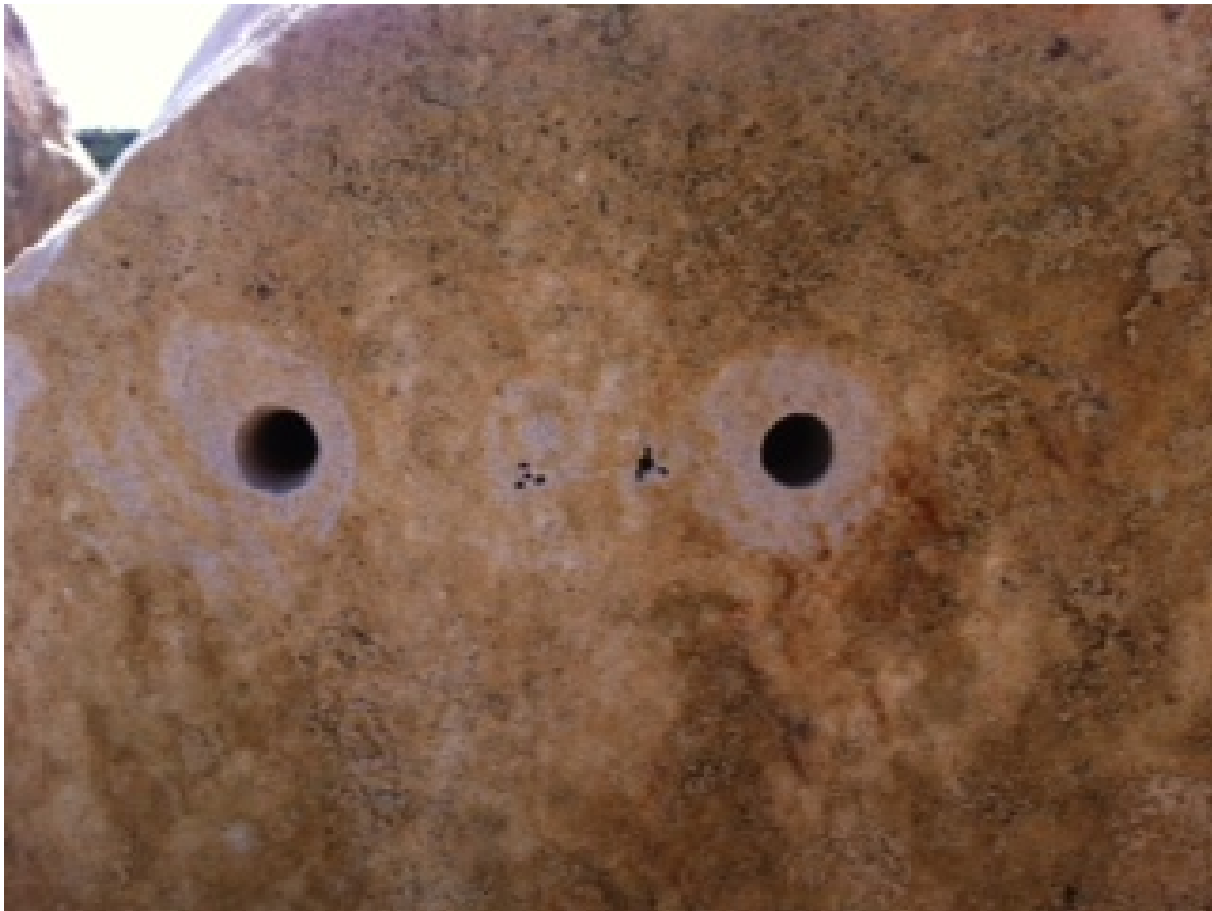
figure 10: Bad Bentheim/Gildehaus sandstone, comparison of boreholes rotating (left and right) and static nozzle design (middle)
