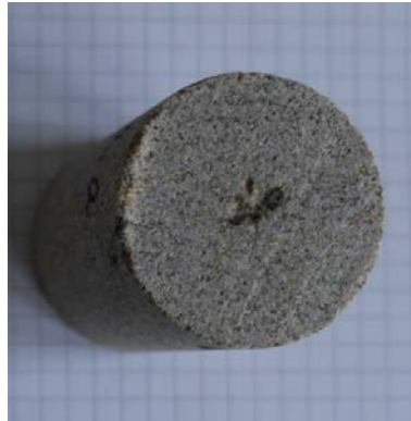
figure 20: Dortmund sandstone after 2:00 min jet exposure time, unsaturated
