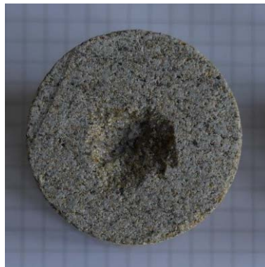
figure 21: Dortmund sandstone after 1:00 min jet exposure time, saturated
