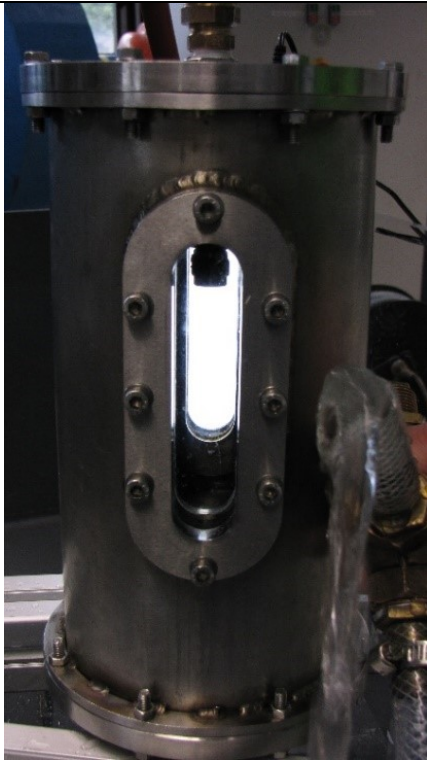
figure 32: pressure cell with single nozzle
