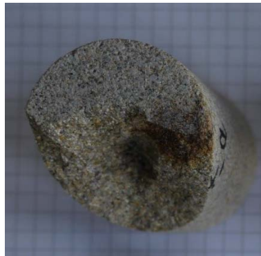
figure 22: Dortmund sandstone after 2:00 min jet exposure time, saturated
