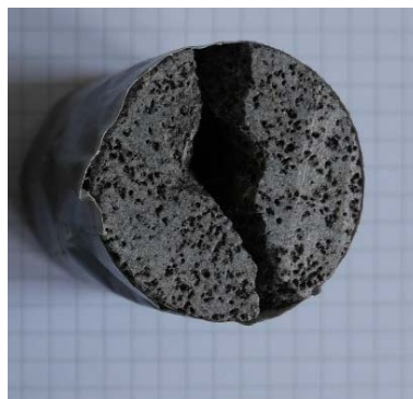
figure 19: Iceland Basalt specimen VBA6-IC-04 at 400 m/s nozzle exit speed
