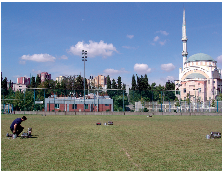
Fig. 3: Top) Array installation in a site in Istanbul. Bottom) Inversion results and fit to the dispersion and H/V ratiion curves (insets) for the array. The figure shows tested models (thin gray lines), the minimum cost model (black line), and the models lying inside the minimum cost model +10% range (thick dark gray lines). Top inset show the observed phase velocities (black line) and the phase velocities for the minimum cost model (gray dots). Bottom inset show the average observed H/V ratio (black line) and the H/V ratio for the minimum cost model (gray dots).
