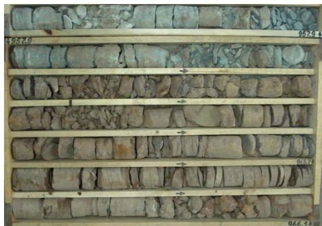
Fig.18. Transition of the grey and red coloured shales, Kemeris formation, well Vydmantai-1. This colour transition can be prognosed in Klaipėda wells in the upper part of the Shale E and continues down to the bottom of the Kemeris Fm. (including Sandstone IV)
