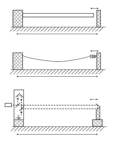
**Figure 1** Schematics of the most frequent strainmeter designs. From top to bottom: rod-, (tensioned) wire- and laser strainmeters. The top two must be equipped with displacement transducers at the right. The bottom sketch indicates the laser, two beam splitters, one corner cube reflector and some sensor (symbol of photodiode) able to detect the change in the interference fringes due to the relative motion of the corner cube reflector on the pedestal to the right.
