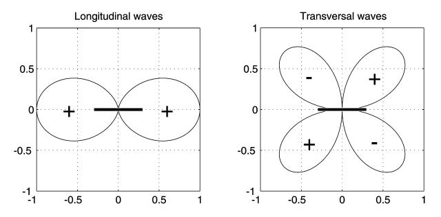
**Figure 3** Relative direction sensitivity of linear strainmeters to apparent longitudinal (left) and apparent transversal (right) elastic waves. The strainmeter is indicated by the thick horizontal bar in the center of diagrams. Note that in both cases the strainmeter response is identical for opposite arrival directions.
