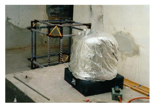
**Figure 5** The whole installation is wrapped with a reflective foil which can be obtained as a part of first-aid kits. The reflective foil reduces radiative and convective heat transport and therefore is part of the thermal insulation. Again it is recommended to extend the foil over the gabbro plate down to the surface of the pier. Ensure that no air-draft can pass underneath the foil. Tape it to the pier or put some heavy items on its edges.
