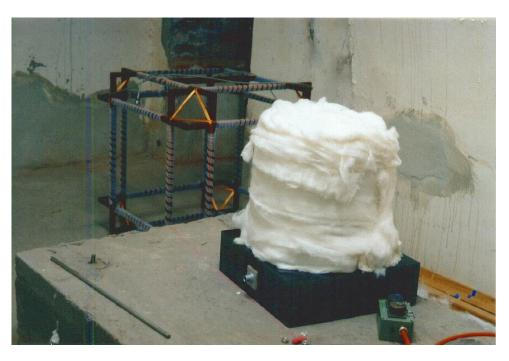
**Figure 4** A second layer of stuffing or fleece is wrapped around the steel container. Other than in this picture it is recommendable to wrap the gabbro plate too. The fleece again serves as a thermal insulation and prevents air drafts from acting directly on the surface of the instrument. Synthetic stuffing fleece with stronger fibres is preferable for this outer layer. The stronger fibres are able to maintain the structure of the fleece even when exposed to high humidity.
