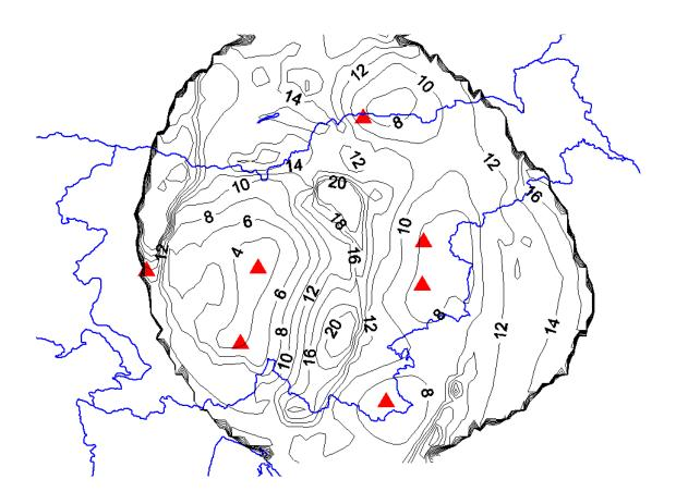
**Figure 1** Result of model calculations for the Stareslo network in Slovenia for Ml = 1.0 earthquake. Red triangles: station positions, blue lines: borders of Slovenia, thin black lines: isolines of hypocenter location error in km; thick black outer boundary: outer limit of the network's location capability for earthquakes of Ml = 1.0.
