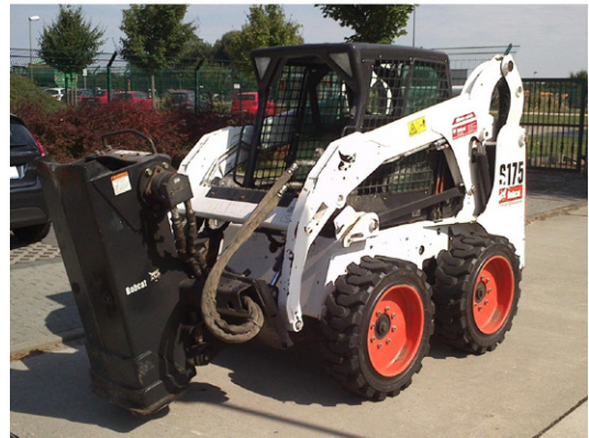
Fig. 3. Photos of the three sources used in this study. A). Vibsist 3000 B). Vibsist 500 and C). Bobcat with drop hammer.
