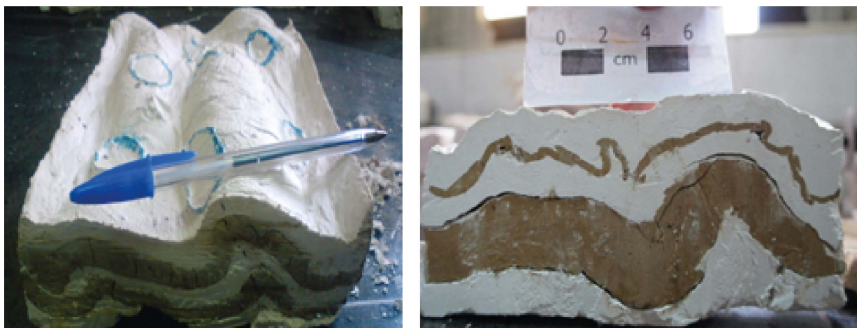
Fig. 4.: Harmonic(a) and polyharmonic folding (b).
