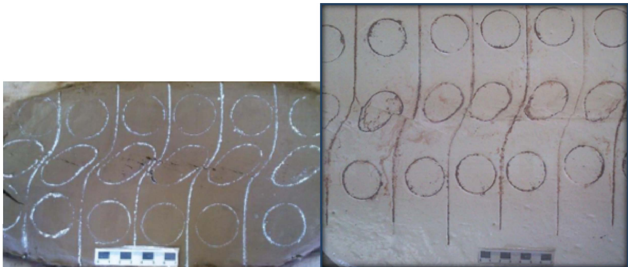
Fig. 6.: Showing the greater development of fractures in wet clay than wet gypsum.
