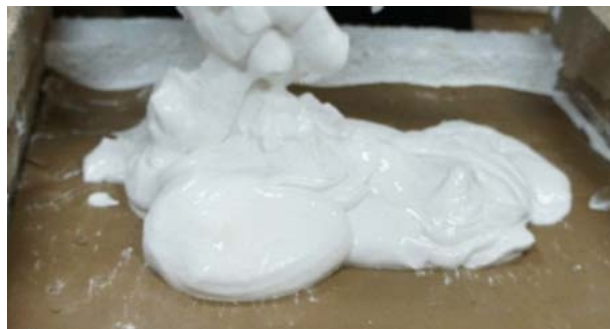
Fig. 1.: Wet gypsum as ductile material in physical modeling.
