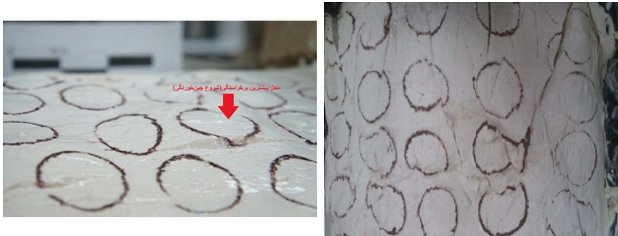
Fig. 5.: development of tensile and shear fractures in wet gypsum.
