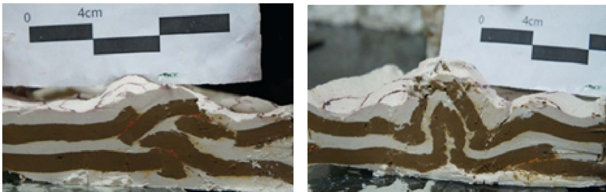
Fig. 3.: The effect of wet gypsum to act as detachment horizon during folding.
