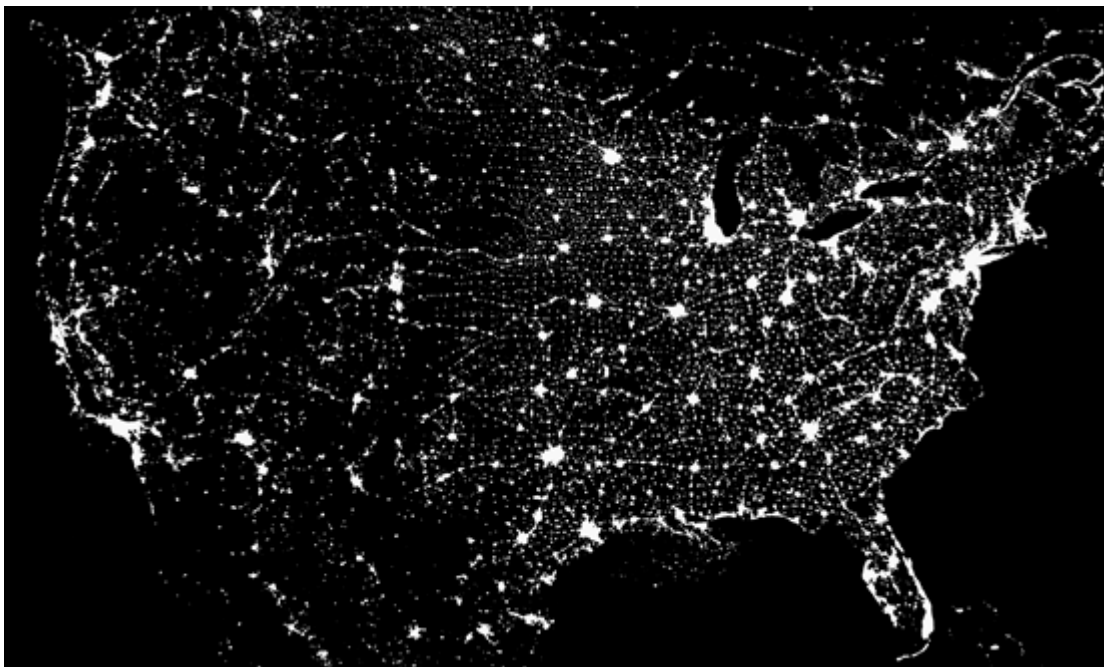
281 282 Figure 8: NGDC’s first map of DMSP nighttime lights, produced from 29 orbits and no 283 cloud screening. 284
