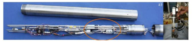
Figure 4-a) Muschong pump installed in the borehole tool for water removal, b) Custom made Muschong pump
