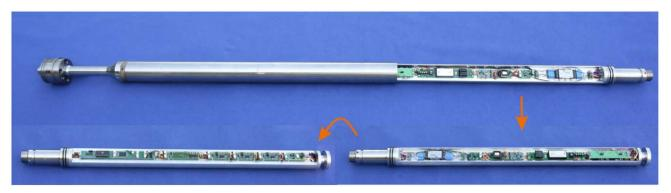
Figure 7—Picture of the telemetry unit in and outside the casing of the borehole tool.
