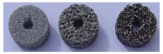
Figure 8—Open-cell aluminum foams with different pore sizes
