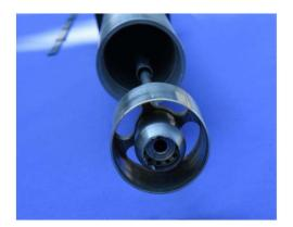
Figure 6—Gas mixing chamber inside the borehole tool. (catalyst bed is not shown.)
