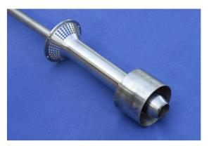
Figure 3—Picture of the water trap.
