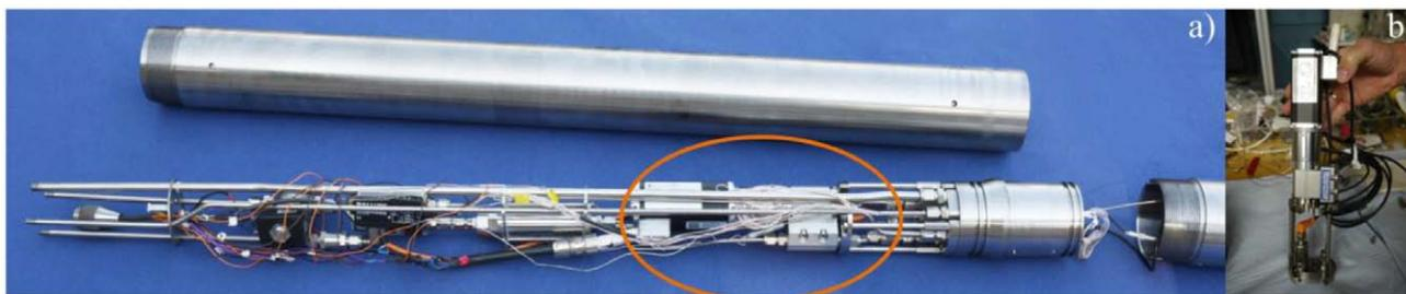
Figure 4—a) Muschong pump installed in the borehole tool for water removal, b) Custom made Muschong pump
