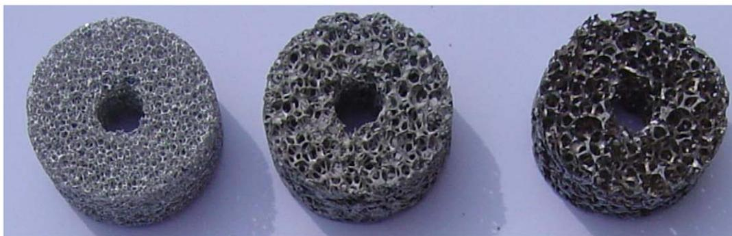
Figure 8—Open-cell aluminum foams with different pore sizes
