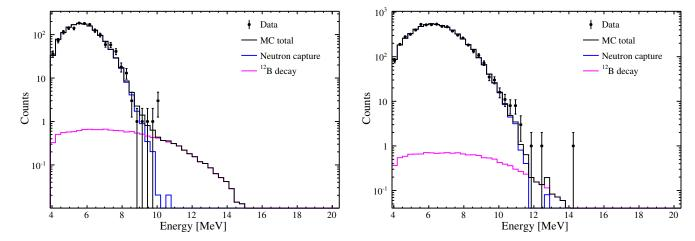
FIG. 5. Determination of <sup>12</sup>B contamination, in Phases I (left) and II (right). The time delay and reconstructed energy (shown here) distributions are fit to a combination of exponentials, corresponding to neutron captures and <sup>12</sup>B decays.
