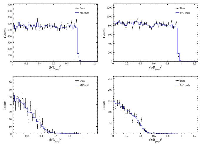
FIG. 6. Area-normalized impact parameters  $b^2/R_{PSUP}^2$  of all muons (top) and only muons with followers (bottom), in Phase I (left) and II (right).  $R_{PSUP} = 850$  cm is the radius of the PSUP. The AV boundary is at abscissa value  $\approx 0.5$ .
