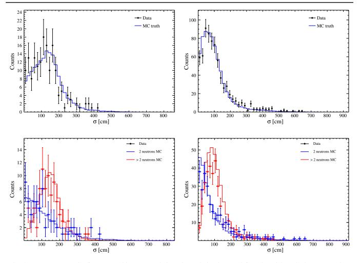
FIG. 10. Per-muon spreads of capture position measured along the track, in Phases I (left) and II (right). The bottom row shows contributions from muons of different multiplicities.
