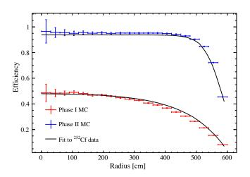
FIG. 13. Low energy capture efficiencies as calculated by simulating <sup>252</sup>Cf-fission neutrons with GEANT4, compared with analytic fits performed to <sup>252</sup>Cf calibration data taken during Phases I and II.
