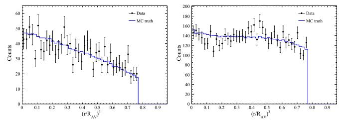
FIG. 9. Volume-normalized capture position  $r^3/R_{\rm AV}^3$  of detected followers, in Phases I (left) and II (right).  $R_{\rm AV}=600$  cm is the radius of the AV.
