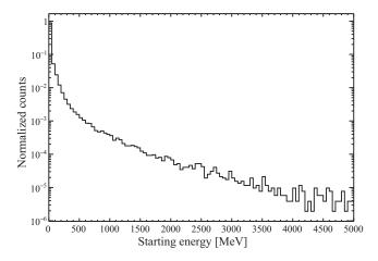
FIG. 2. The spectrum of starting energies of muon-induced neutrons at SNO, as generated by GEANT4.
