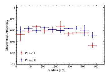
FIG. 4. SNOMAN-based observation efficiency for neutron captures on D in Phase I (red), and <sup>35</sup>Cl in Phase II (blue). Error bars are statistical.
