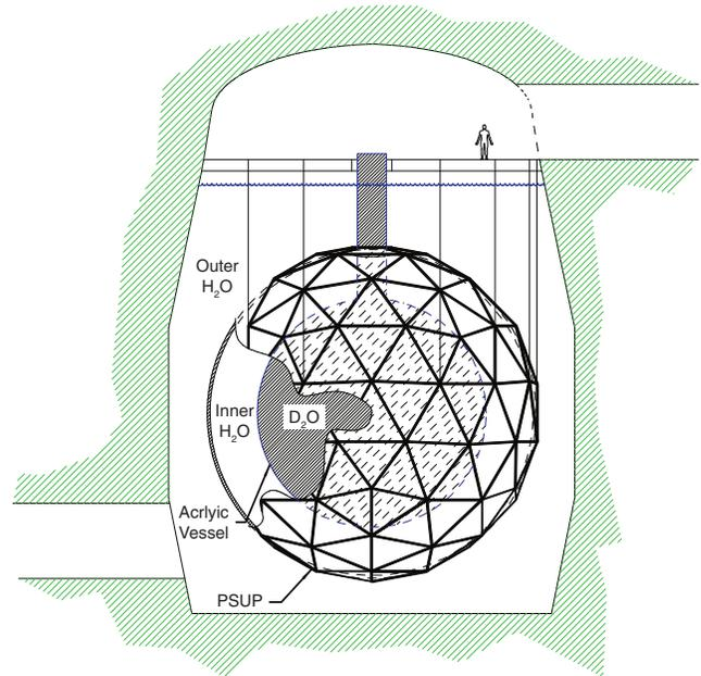
FIG. 1. Schematic diagram of the SNO detector.
