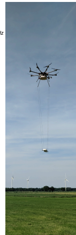
Photos: The System includes 2 miniaturized OPM Sensors arranged in reversed orientation. Averaging of sensor data allows to reduce the heading error significantly. The DJI s1000+ achieves ~18 min flight endurance with the MagArrow bird suspended as payload.
