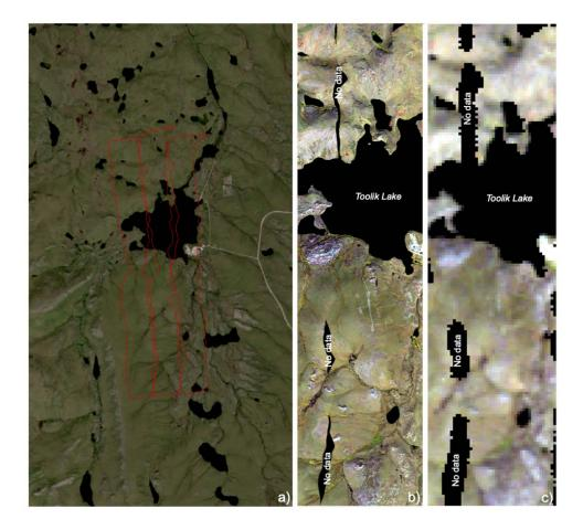
Figure 2 a) Sentinel-2 image (06.07.2016) overlaid with the three flightlines used to create the orthomosaic, b) Orthomosaic of the AISA flight lines clipped to the general area where ground-based data were collected. c) Simulated EnMAP orthomosaic generated from the AISA data. Black areas marked with No data are the result of non-overlapping flight lines. Black areas not marked with No data are water bodies. Imagery courtesy A Beamish and (Beamish, 2018)
