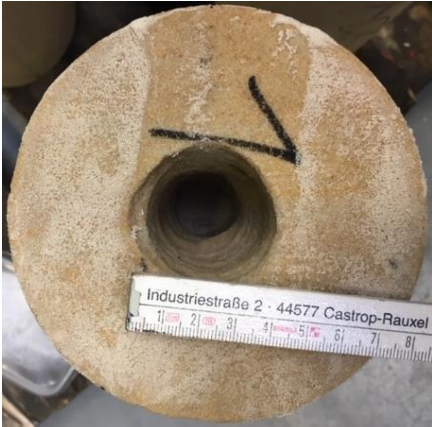
figure 19: Gildehaus sst, lateral created by rotating nozzle StoneAge© Beetle tube spinner
