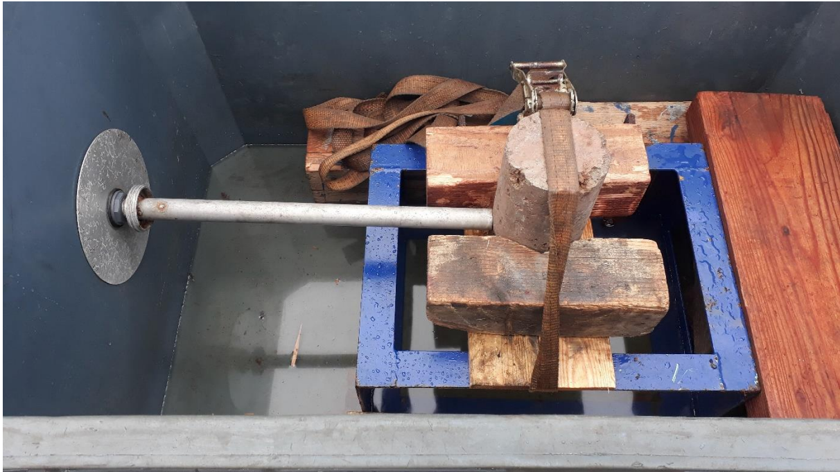
figure 44: Rock sample firmly attached to the guiding tube with nozzle inside. Additionally the sample is strongly tied to the metal frame beyond
