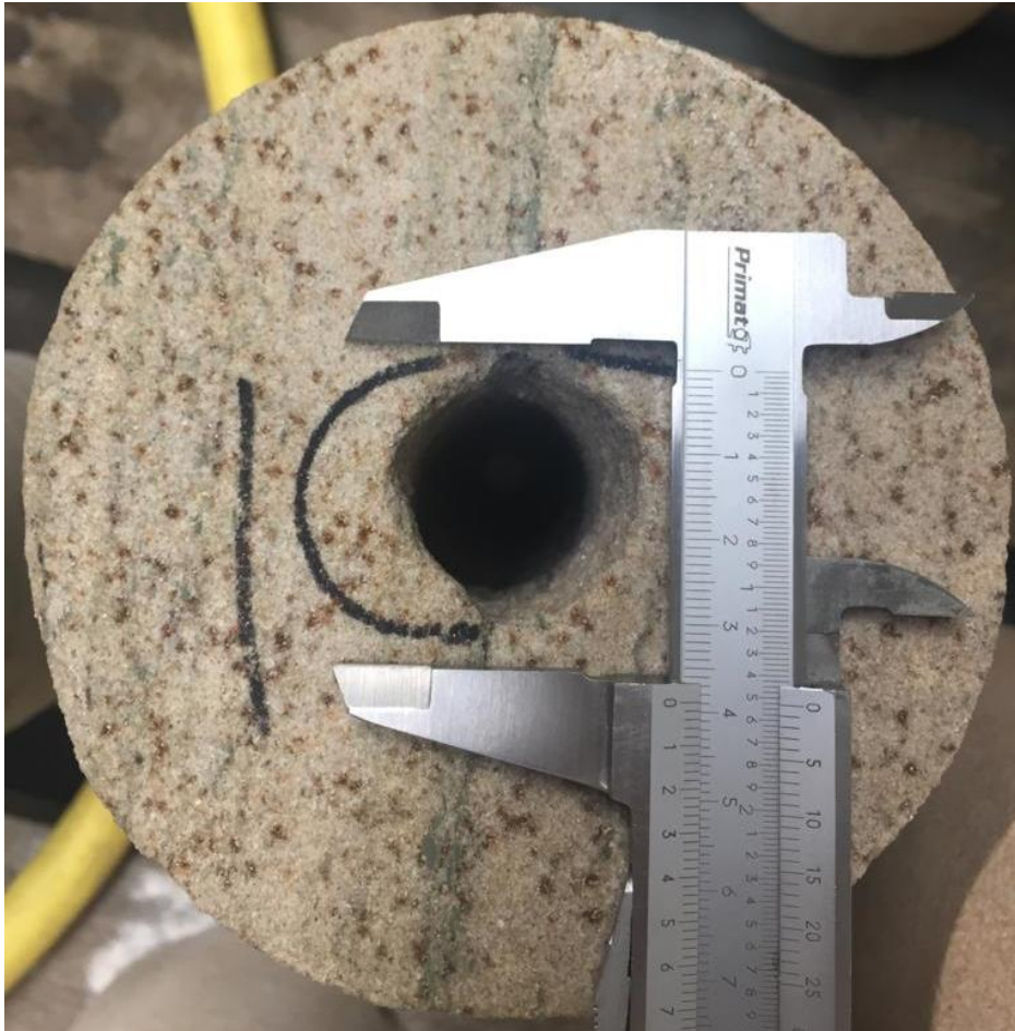
figure 21: Friedewald sst, lateral created by rotating nozzle design
