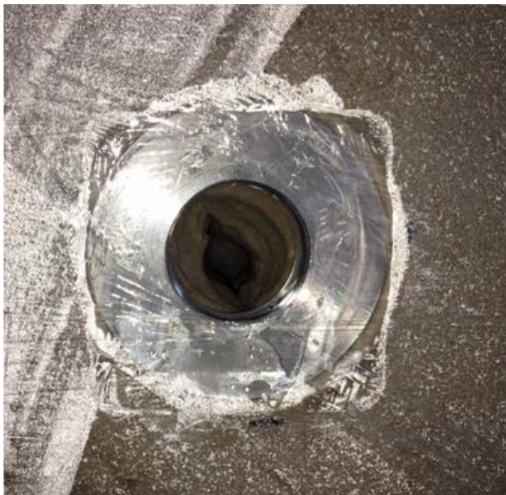
figure 30: thread connection in rock specimen for steel pipe
