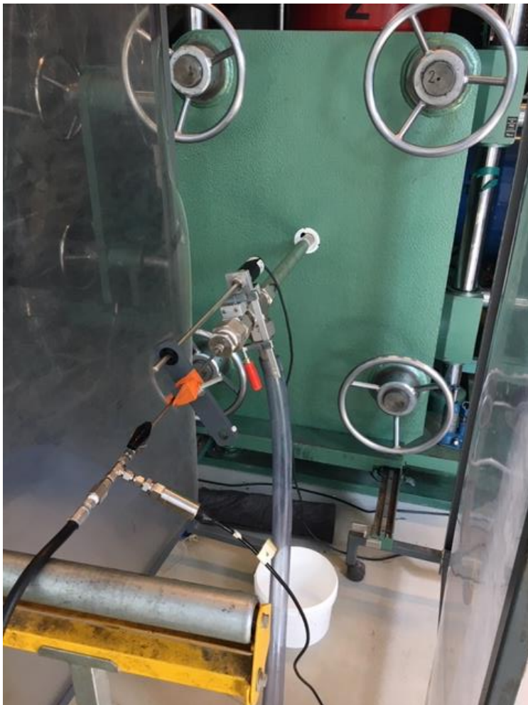
figure 29: photo of tri-axial cell front plate and connected steel tube
