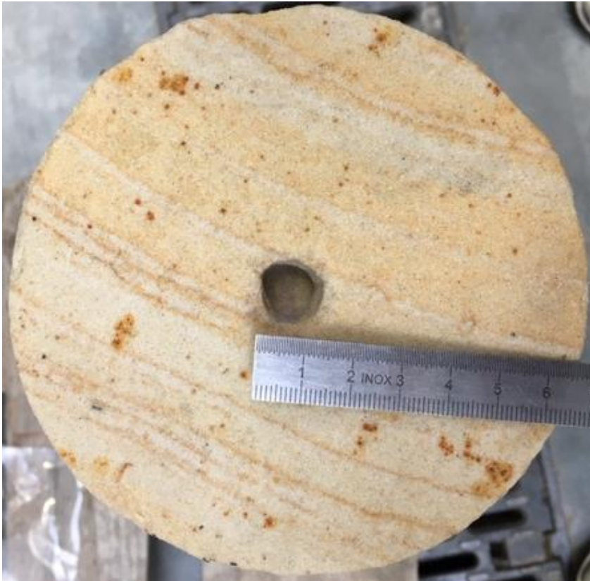
figure 17: Gildehaus sst, photo of cavity by static nozzle design of WSG
