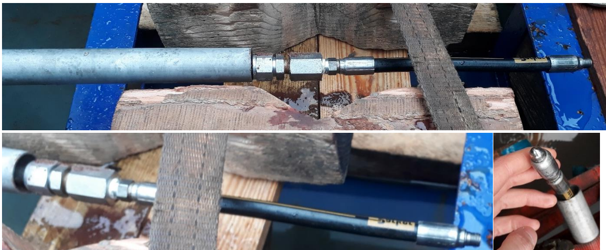
figure 45: HP-pipe with flexible hose and threaded connection for a nozzle at its end guided with little radial clearance inside the outer tube
