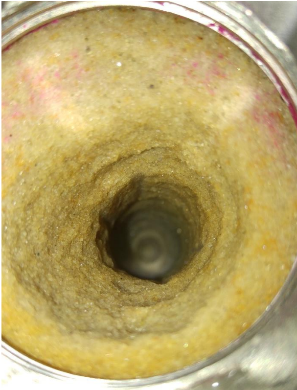
figure 35: lateral shape after jetting experiment with GI-03
