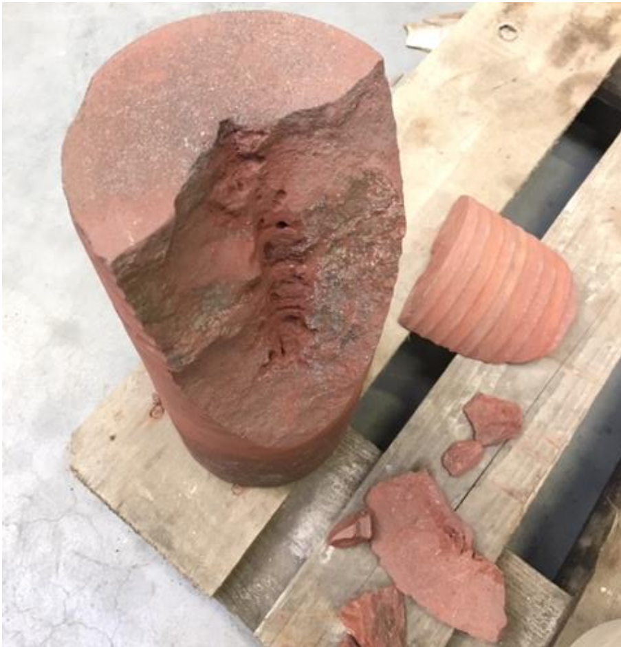
figure 22: Iceland sedimentary layer, fractured specimen after test using rotating nozzle design
