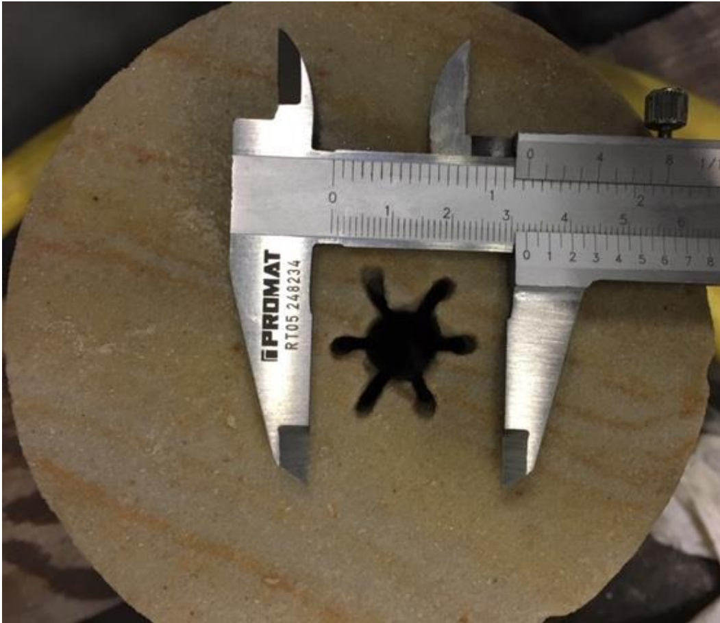
figure 18: Gildehaus sst, star shape borehole by static nozzle of Buckman© nozzle design
