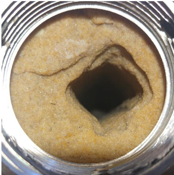
figure 37: lateral shape after jetting experiment with GI-04
