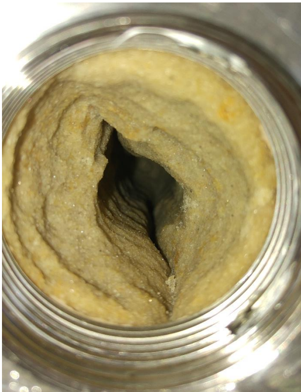
figure 33: lateral shape after jetting experiment with GI-02
