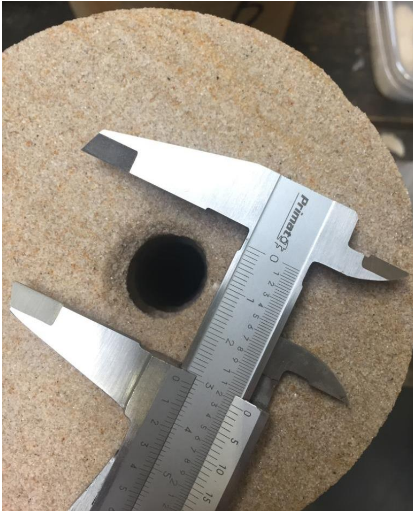
figure 20: Bad Dürkheim sst, lateral created by rotating nozzle design
