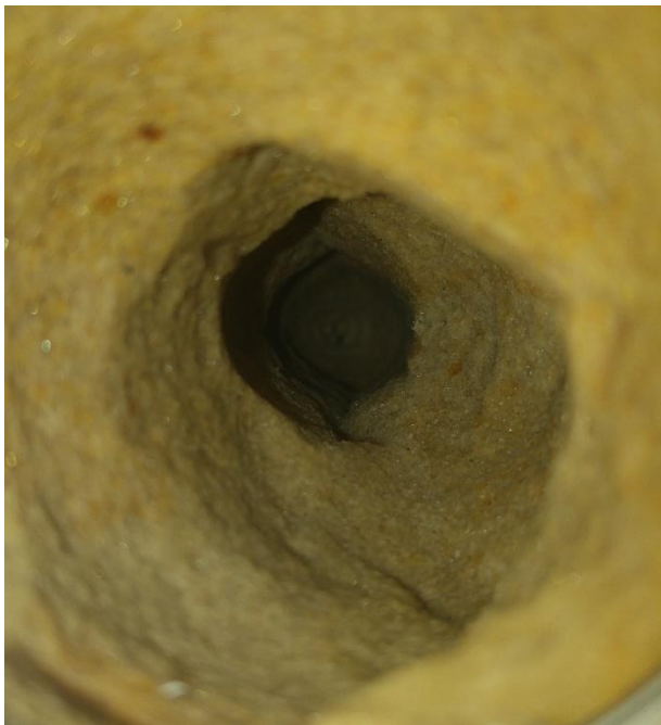
figure 41: lateral shape after jetting experiment with GI-06
