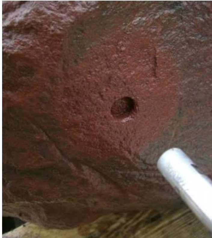
Figure 5. Sample of inter-basaltic sedimentary layer jetted at HBO/GZB in Bochum (picture: HBO/GZB).
