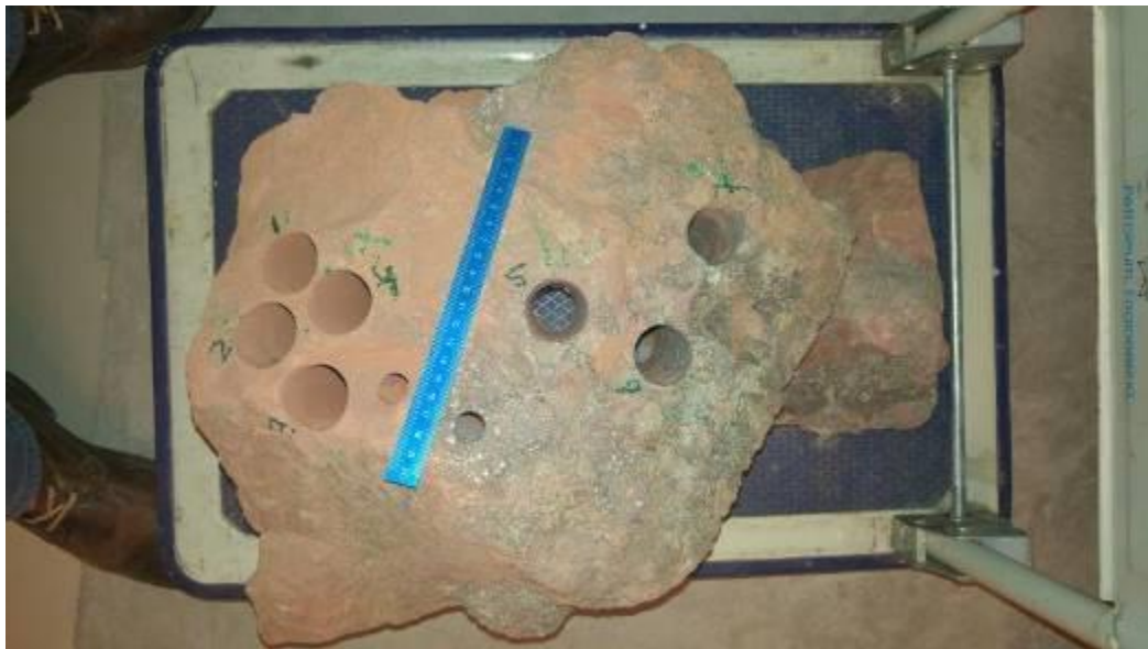
Figure 6. Sample locations used for mechanical testing. Picture by TUD/GFZ.
