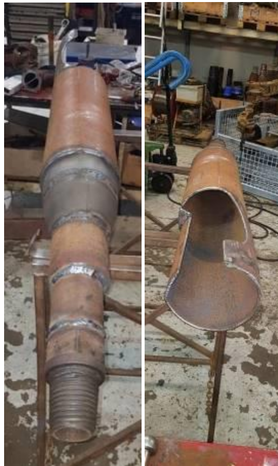
Figure 43. Raekto's custom made overshoot built around a sub with NQ threads used for second fishing trial (figure by Raekto).
