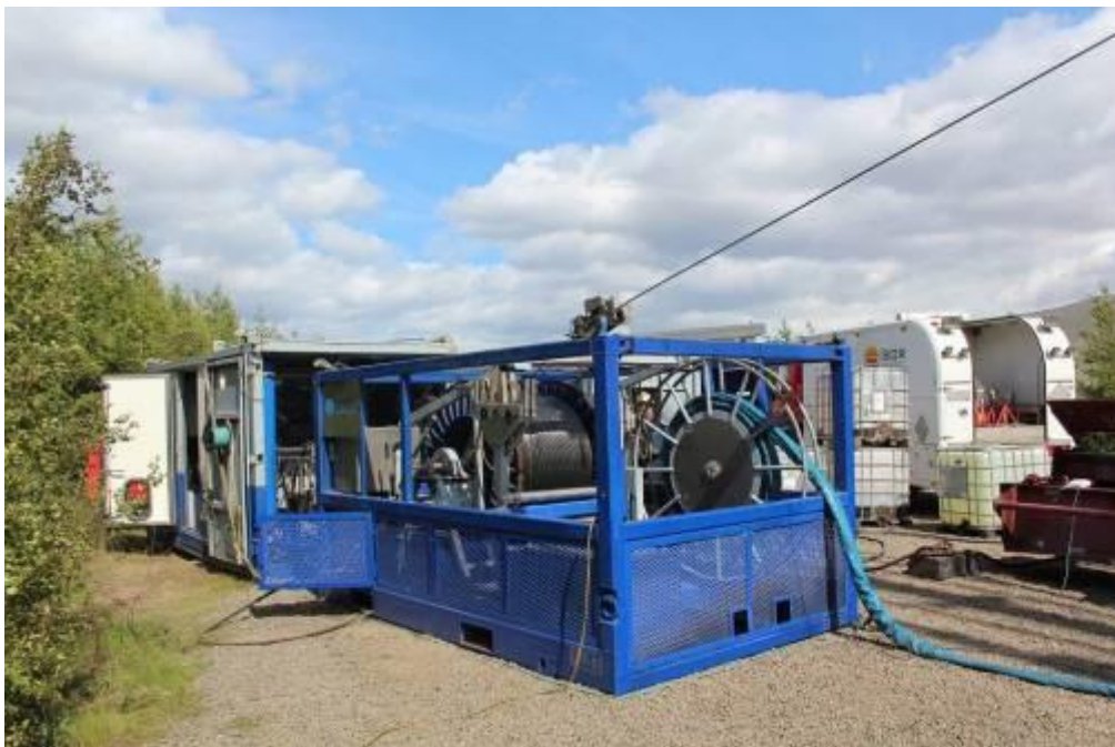
Figure 46. WSG's coil unit and control unit (picture taken in June 2019 during RJD).
