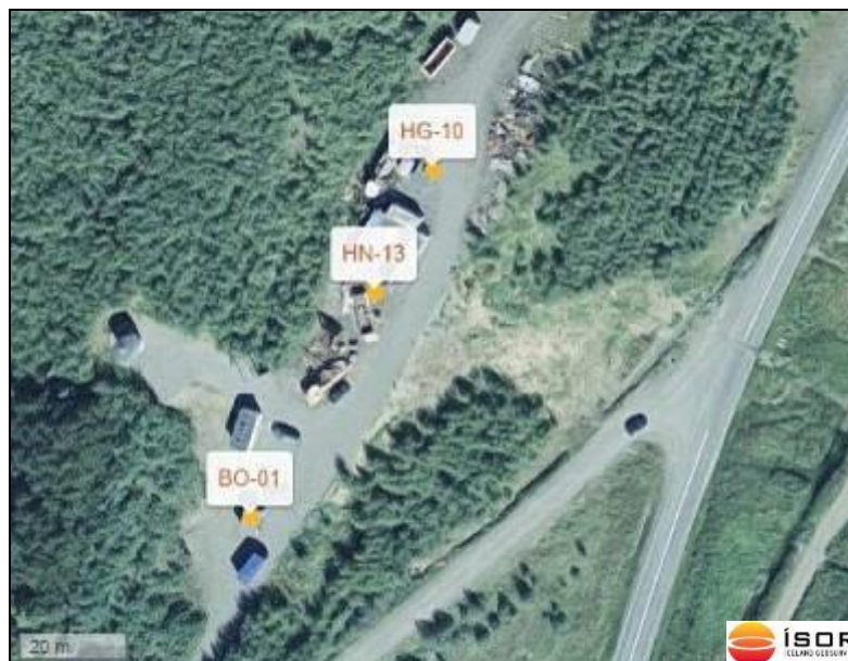
Figure 18. Drillpad of HN-13. The well sits in the middle of the drillpad, that is 20 m wide and 80 m long.
