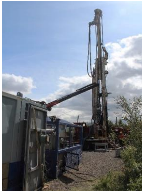
Figure 47. WSGs coil and control unit running in hole through injector held up by a crane (picture taken in June 2019 during RJD).
