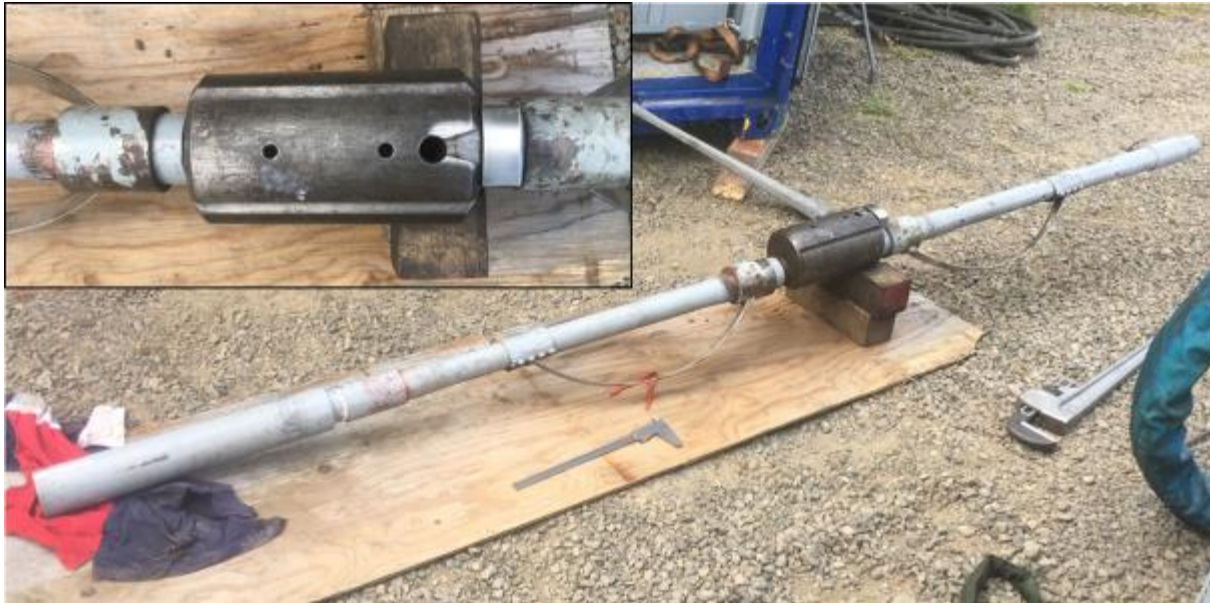
Figure 45. BHA consisting of de-centralizers and a deflector shoe (pictures by WSG onsite in June 2019).
