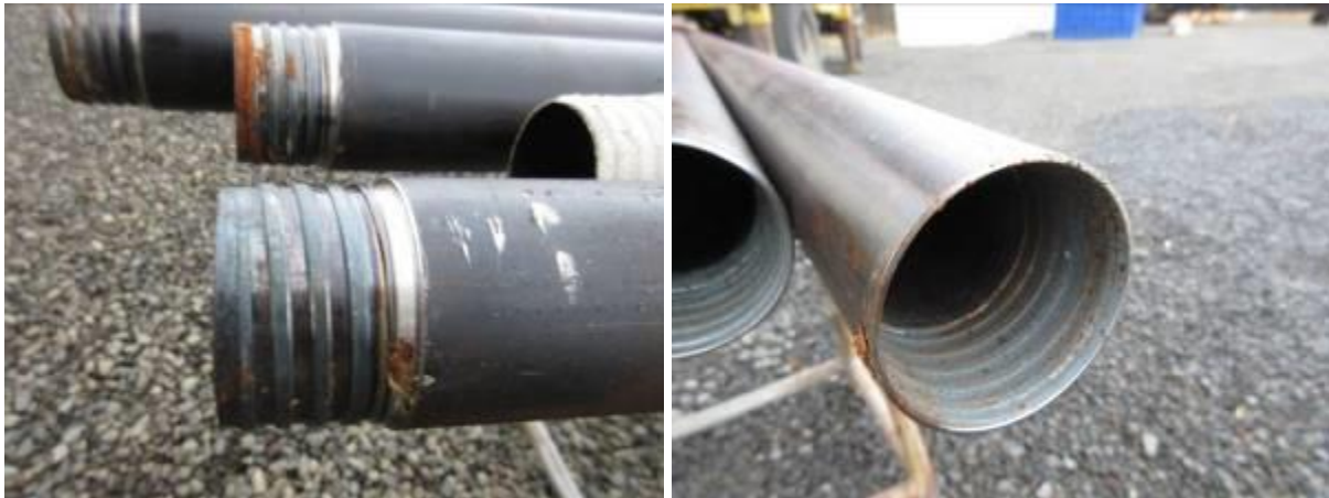
Figure 42. Drillpipes used for deploying deflector shoe. This type (NQ) of drill pipes is normally used for coring and is lighter than usual drill pipes and are flush, i.e. the outer diameter is the same for the pipe body and the connection.
