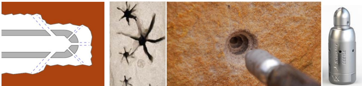
Figure 1. RJD holes and nozzles: Left to right: principal of forward and backward thrusters in static nozzle; star-shaped profiles in soft limestone with unconfined rock and static nozzle; conical stop-start geometries formed at head of rotating nozzle; detail of Beetle, BT 18 mm rotating nozzle available from “StoneAge” used in true-triaxial laboratory tests performed at TUDelft by Richard Bakker (TUDelft) and Simon Hahn (GZB) in WP4 and WP5.
