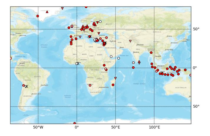
Fig. 1: GEOFON stations in 2018. Colours denote the data availability (white: 0% to red: 100% availability). Symbols represent the level of maintenance needed: circle for "none", square for "on site", triangle (up) for "remote", triangle (down) for "Remote including HW shipment". An "X" next to the symbol indicates metadata updates.
