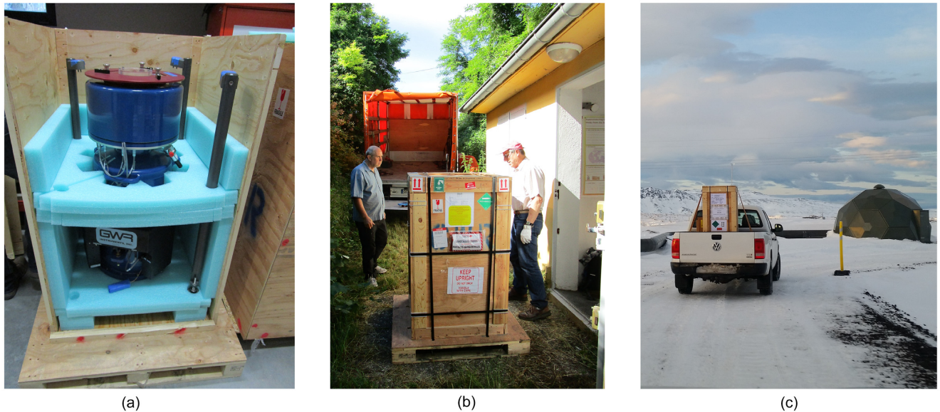
Figure A4. Packing and transport of the iGravs with liquid helium filled (4 K, cold transport); after securing the Dewar and component parts inside the GWR supplied crates (a and b at J9, Strasbourg), the instruments were transported by truck and ship freight to the remote monitoring sites in Iceland (c).
