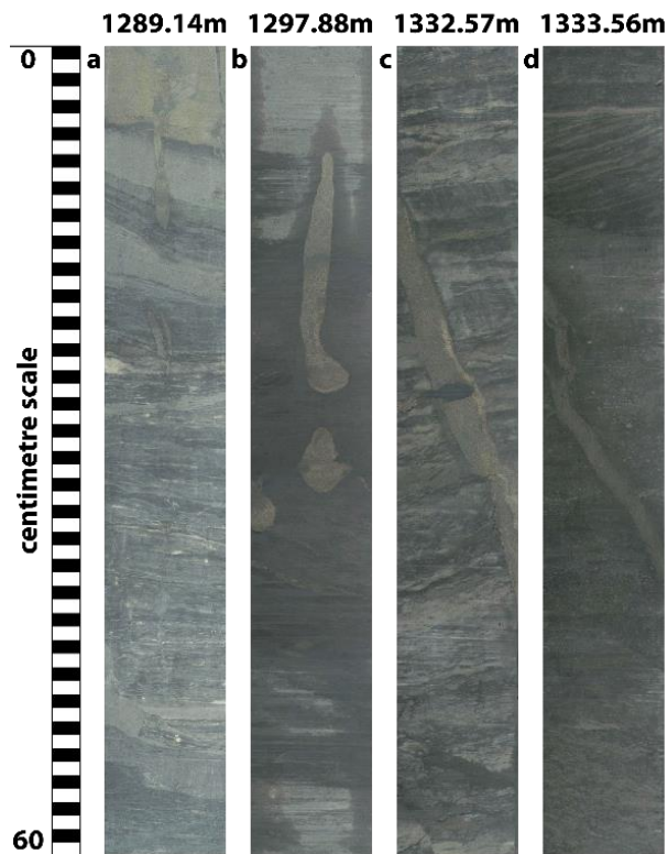
Figure 12 Selection of core photographs that show sandstone intrusions into the mudstone caprock of well B20 of (a-b) vertical break-through and (c-d) fracture-associated types. Depth in metres below mudline. See Figure 14 for stratigraphic context.
