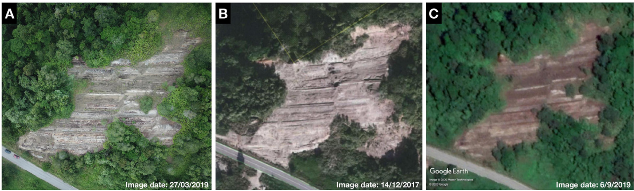
Figure 4: Comparison of aerial images of the “Lion King” outcrop in Jerudong ( 4^{\circ}53'36.25''\text{N} , 114^{\circ}49'59.01''\text{E} ): (A) DJI Mavic Pro (resolution: 4000 \times 3000 pixels); (B) Ortho-photo obtained from Survey Department, Ministry of Development, Brunei (resolution: 1085 \times 715 pixels); (C) Satellite image obtained from Google Earth Pro (2019) (resolution: 1175 \times 758 pixels). The images from the DJI Mavic Pro produce much clearer and sharper details.
