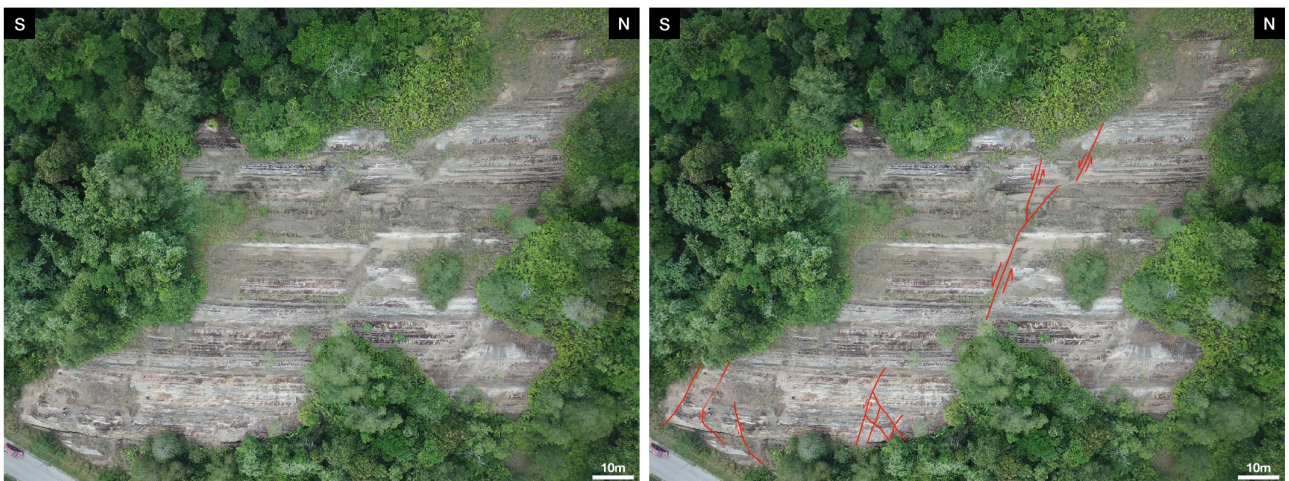
Figure 3: The high-resolution image (4000x3000 pixels) shown on left was captured by the drone, DJI Mavic Pro, and it shows high image quality with clear evidence for faulting (right side) at the "Lion King" outcrop in Jerudong, which is one of the best outcrops to study the faulted sedimentary rocks in Brunei.
