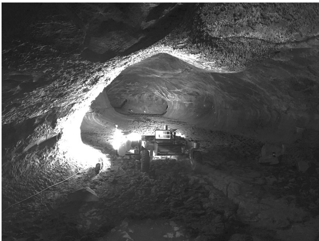
FIG. 2. The NASA Ames K-Rex testing robot, renamed CaveR (“Cave Rover”) for its deployment in a volcanic cave at Lava Beds National Monument in northern California. Here, CaveR is shown moving in the down-flow direction inside Valentine Cave, scanning one side of the cave wall. Attached to the rover is a rectangular instrument pod, housing lamps, cameras, and spectrometers that were used to interrogate the cave wall during a Mars mission simulation that was a component of NASA’s BRAILLE project. In the future a system like this could be used to explore caves on Mars (shown by Blank, 2019 abstract 5108).
