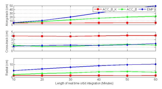
**Figure 10.** RMS values of LEO orbits for the along-track, cross-track, and radial direction for every 10 min over a one hour period.
