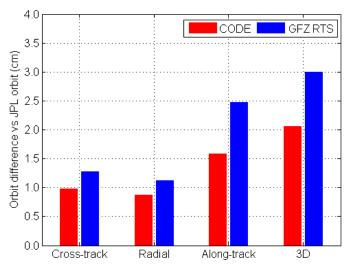
**Figure A2.** RMS of GRACE-C orbit with respect to JPL PSO orbits by using CODE final products and GFZ real time products.
