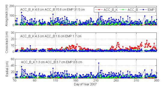
Figure 7. Averaged RMS values for the three directions with three strategies for an orbit prediction of one hour.
