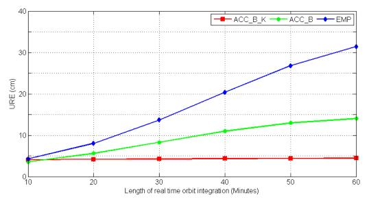
Figure 11. URE for every 10 min over a one hour orbit prediction.
