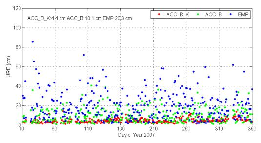
Figure 8. User Ranging Error (URE) of a real time LEO orbit for three different strategies.
