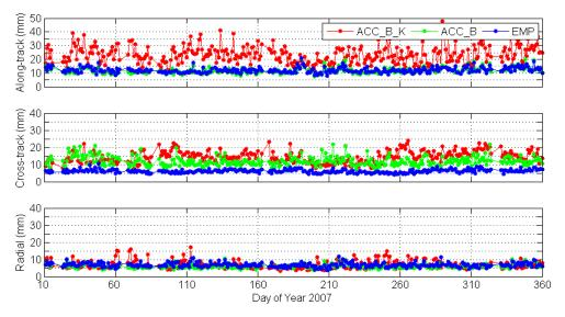
**Figure 3.** Averaged Root Mean Square (RMS) values for along-track, cross-track, and radial directions with the three strategies.
