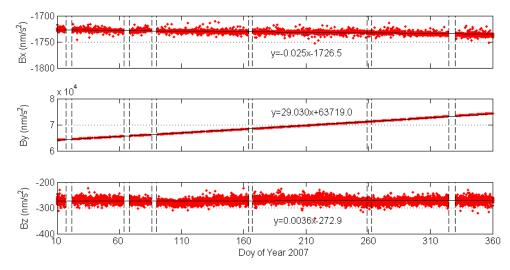
**Figure 4.** Accelerometer bias parameters for strategy 2. The data between black dashed lines are excluded because of the change of the controller onboard or abnormal behavior of accelerometer. Black lines are the linear fitting line. The corresponding fitting results are also shown in each panel.
