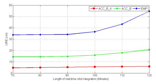
**Figure 12.** RMS values of LEO orbits for the along-track, cross-track, and radial direction for another one hour and corresponding URE values.
