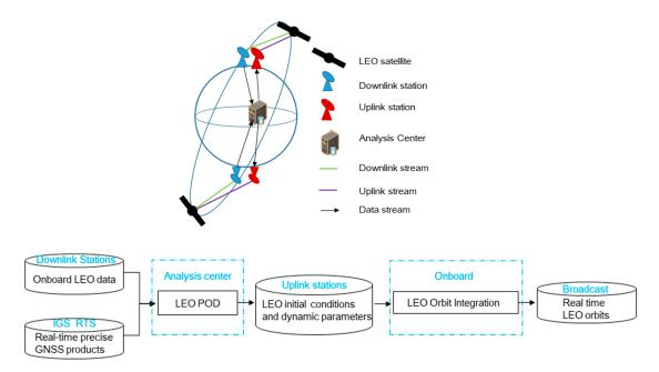
**Figure 1.** Procedures of Low Earth Orbit (LEO) orbit prediction. The LEO onboard Global Navigation Satellite System (GNSS) and accelerometer data are downlinked and transferred to the analysis center and processed there. The estimated initial condition states of LEO as well as the dynamic parameters are then uplinked to LEO satellites and the predicted LEO orbit is integrated onboard.
