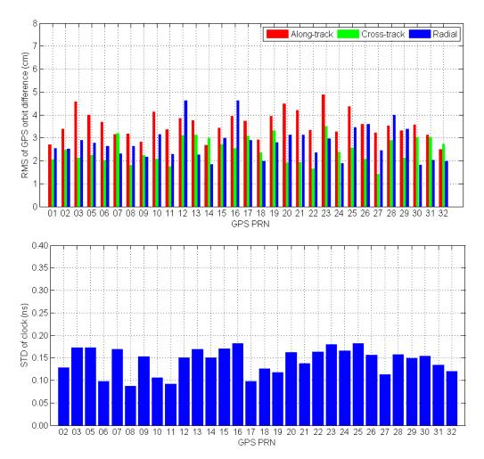
**Figure A1.** RMS of GPS orbit difference (*top*) and STD of GPS clock difference (*bottom*) between CODE products and GFZ real time products.
