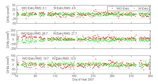
**Figure 5.** Averaged RMS of calibration parameters' differences between using the extrapolated calibration parameters and the estimated ones as well as the averaged RMS of calibration parameters' differences between using the last set of calibration parameters and the estimated ones for each arc. "W/O Extro" means without extrapolated and "W Extro" means with extrapolation.
