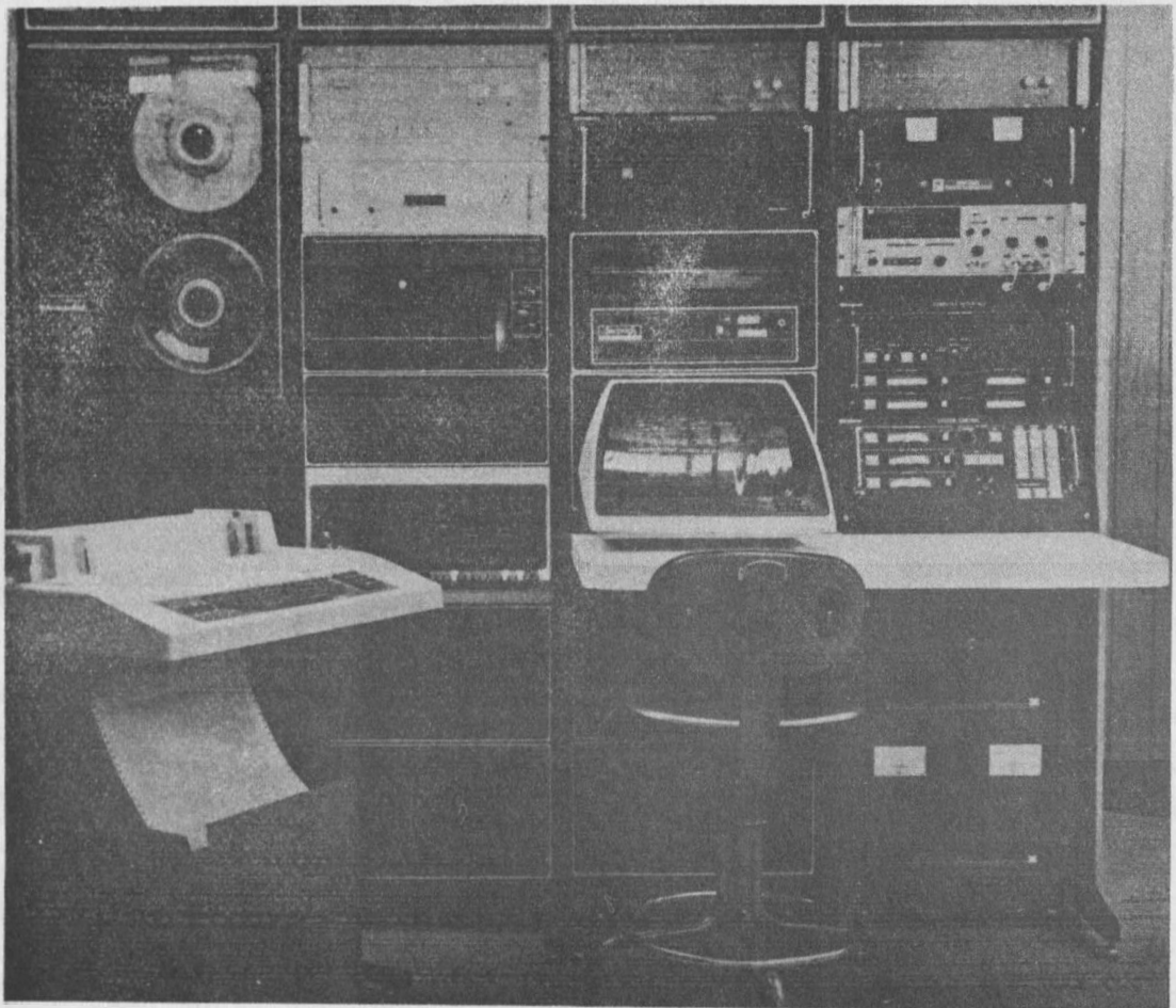
fig. 2: Control unit with PDP-11-45 computer and peripherals, epoch/range counting devices and control interface unit.
