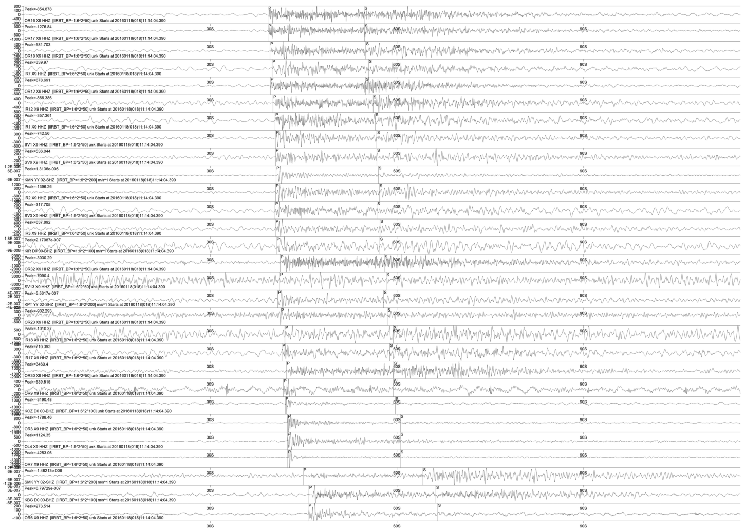
Figure 3. Example of the screenshot of the DIMAS software (Droznin & Droznina, 2011) during the picking of an event occurred on 15 January 2016 at the depth of 150 km. The waveforms in all stations (vertical components) and picked phases of the P and S waves are presented. Note that the S phases were picked based mostly on the horizontal components, which are not presented here.
