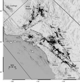
Precisely relocated seismicity in southern California, USA 1981 – 2011
