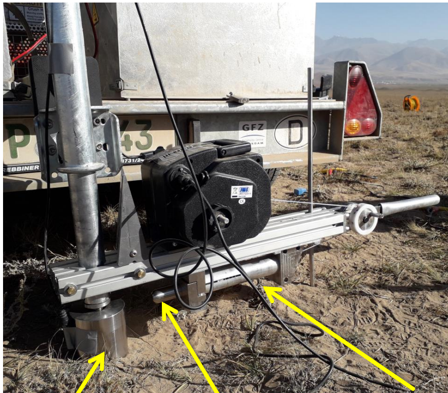
Jacket (with sliding bearings and spring inside)
