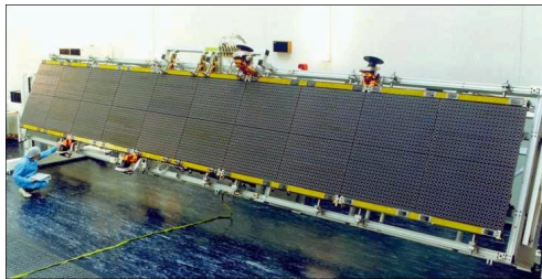
Radar antenna (10x1.3 m), (Photo: ESA)
