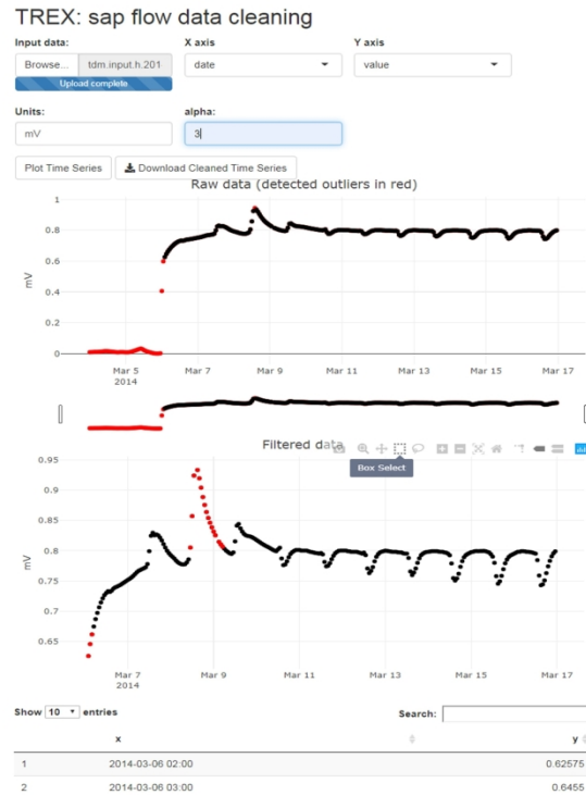
Figure 3. An illustration of the outlier() function, launching a Shiny application for interactive time series visualization and inspection. Users can adjust the alpha parameter for the automatic detection of outliers. Red points in the upper panel highlight the automatically detected outliers, while red points in the lower panel are manually selected points.
