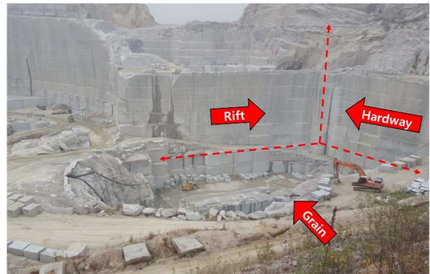
Figure 6. A granite quarry in the Pocheon area of South Korea. The directions of rift-, grain- and hardway planes are indicated by arrows.
