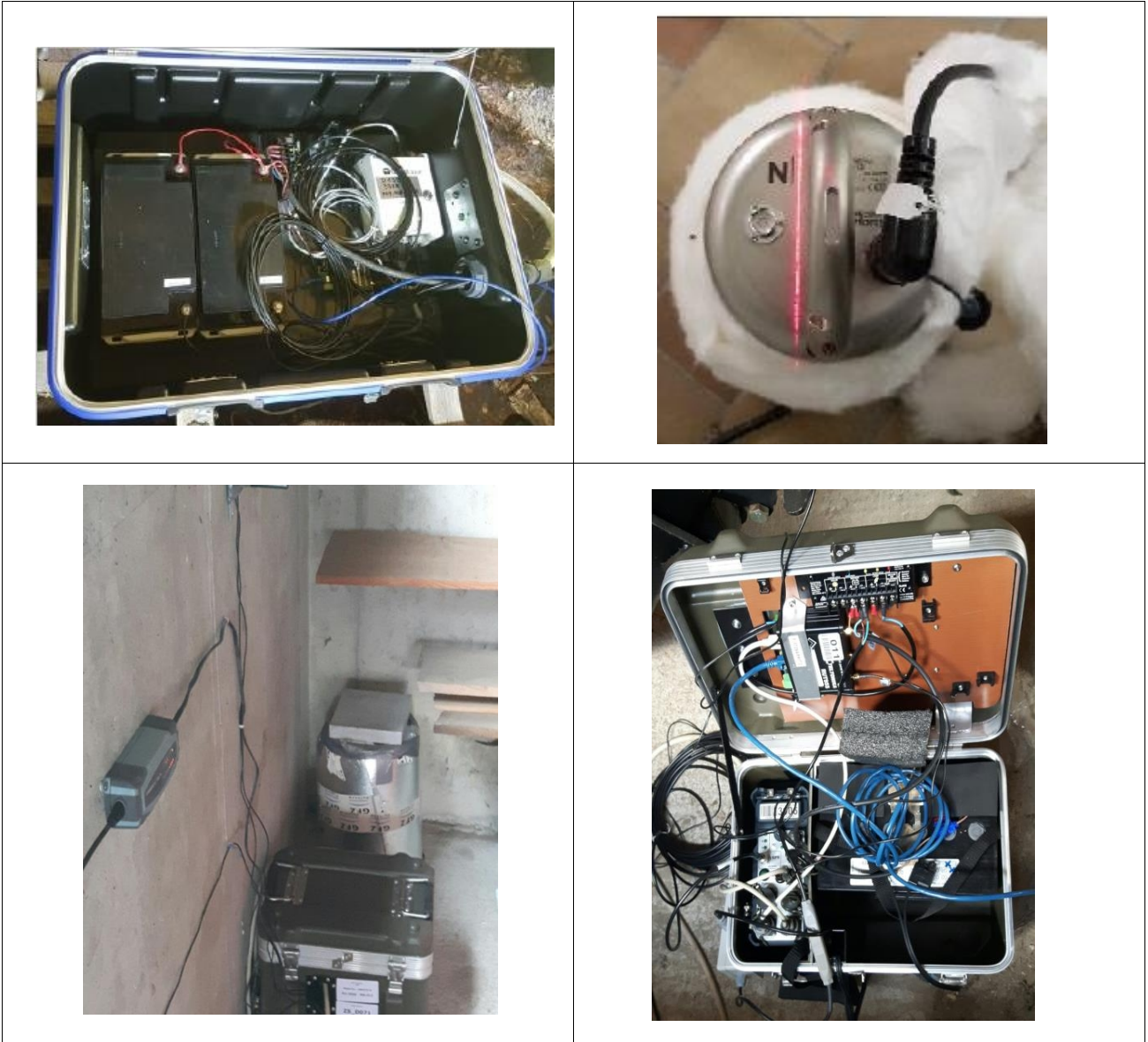
3 Figure 3: Typical installation of a real-time station in a basement. Top left: the green box 4 encloses the datalogger (EDR-210) and the router. The logger is, connected via the white 5 cable with the Güralp seismometer, which is placed below an upturned bucket covered with 6 silver insulation cover (in the background). On the wall the automatic charger (output 12V/DC, 7 5A) controls the trickle charge to the battery. GPS cable connection to the antenna placed
