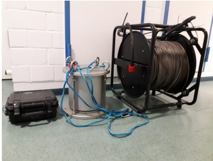
Figure 2: “Mobile Ocean Bottom Seismometer” (MOBSI) system: cable drum (right), broad band seismic sensor & data logger (middle) and control unit/computer (left).
