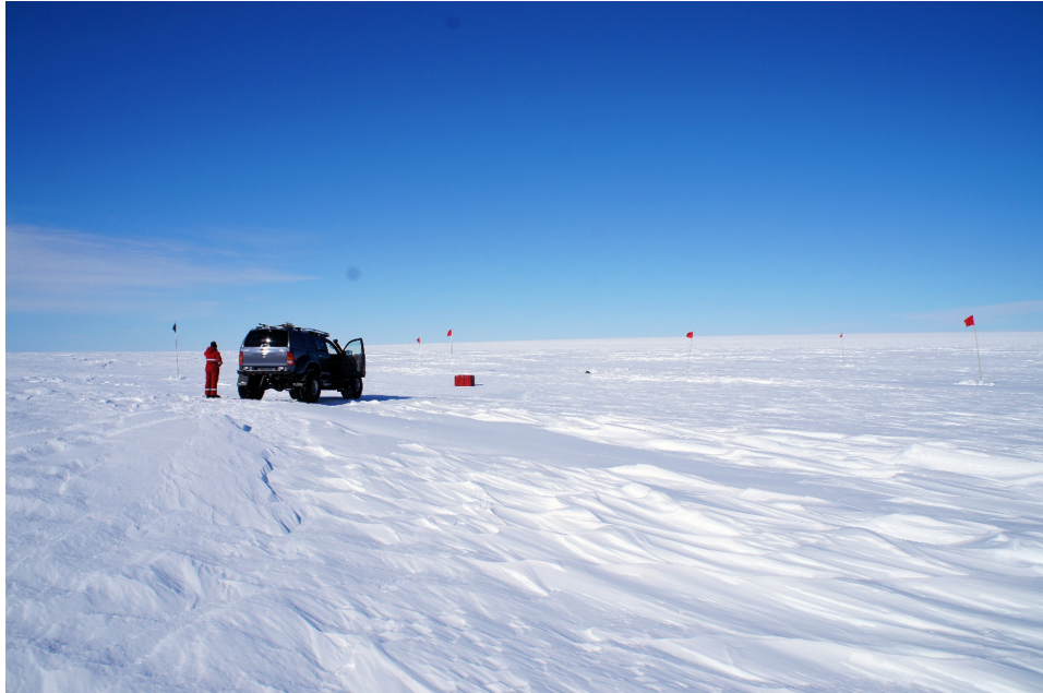
Figure 6: Deployment of magnetotelluric station: After installation, the positions of sensors (electrodes and induction coils) were marked with bamboo sticks. The red box contains the data logger. Typically after 3-5 days of recording all components were recovered and taken to the next station.
