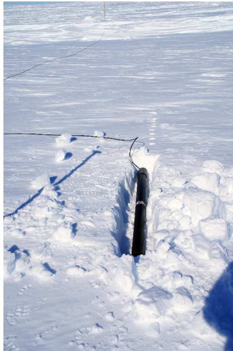
Figure 5: Deployment of magnetotelluric station: Induction coil magnetometers were buried in approximately 50 cm deep holes in the snow. Two of these induction coils were installed horizontally, another one in the vertical direction.
