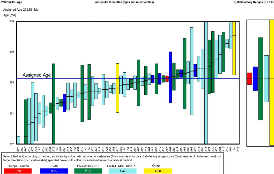
Figure 1: - Distribution of contributed 206Pb/238U age results for G-Chron 2019 in relation to the assigned age, specified target precisions (z = 1) and corresponding satisfactory ranges (z = ± 2) for Rak-17, Zircon
