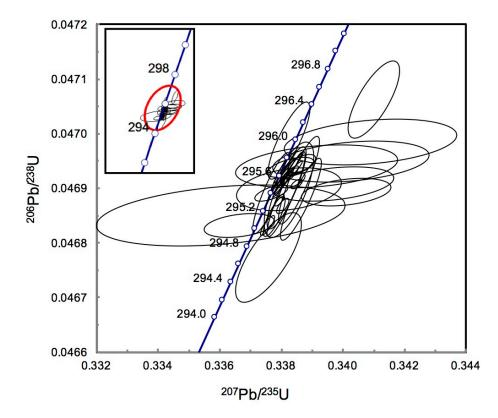
**Figure B:** U-Pb concordia plot for 35 determinations by isotope dilution as reported by seven independent TIMS laboratories. Inset upper left: the same data at a compressed scale along with a red ellipse showing the mean result from the SIMS data (see Figure A). All ellipses represent 1s uncertainties. The concordia curve and age values (in Ma) are based on the decay constants of Steiger and Jäger (1977).
