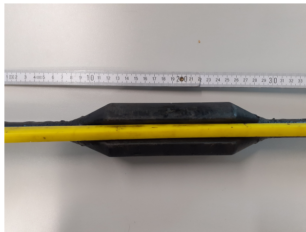
Figure 1. Downhole cable configuration of the sucker rod with a centralizer (black) and the fiber-optic cable (yellow).
