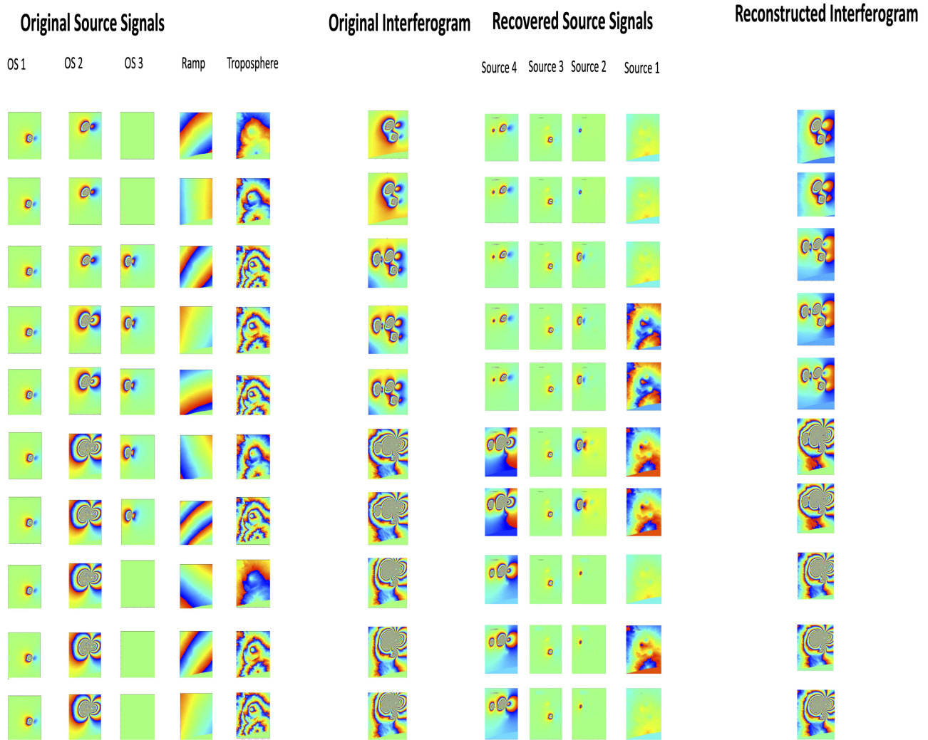
Fig. 7. Figure showing the Mogi source signals OS1, OS2, OS3, the ramp and tropospheric noise signals, the original interferograms, the recovered signals from the algorithm and the reconstructed interferogram from the recovered signals for 10 different simulated interferograms of temporal baseline 33 days.
