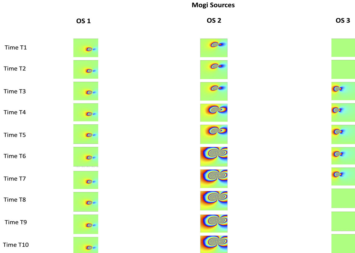
Fig. 3. Temporal nature of three types of Mogi sources considered for time ranges from T1 to T10. OS1, OS2, and OS3 refer to the three types of original Mogi sources: a constant source with a specific constant amplitude throughout entire duration, a temporally increasing source, the amplitude of which increases with time and an episodic source, which has a high amplitude for a brief period of time and then subsides abruptly, respectively.
