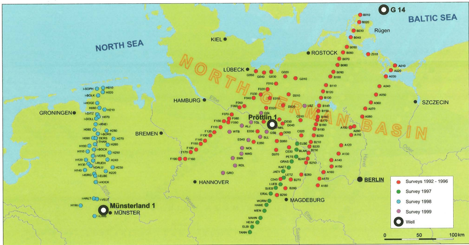
Fig.1: Magnetotelluric sites in the North German Basin
