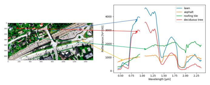
**Figure 2.** At surface reflectance of some urban surfaces (HySpex sensors VNIR-1800 and SWIR-384). The hyperspectral dataset was acquired by the Terratec AS Company in August 2019 over Baerum municipality, Oslo, Norway.
