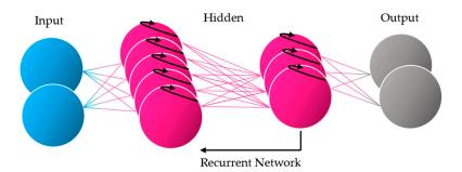
Figure 8. Recurrent neural network architecture.
