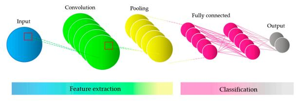
Figure 7. Convolutional neural network architecture.
