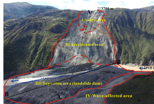
Figure 2: Overviews of the Baige landslide affected area divided into four parts: (I) the source area, (II) the acceleration area, (III) the deposition area, and (IV) the wave affected area (Ref. [70]). The height of deposit along A-A and B-B sections will be compared with numerical results in subsequent analyses.
