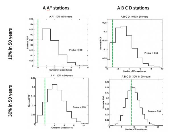
**Figure 9.** Results of the consistency test of MPS19 with the observed PGA values in the last decades for different PoE (10% and 30% in 50 years). The meaning of sites A, A\*, B, C, and D is reported in the text.
