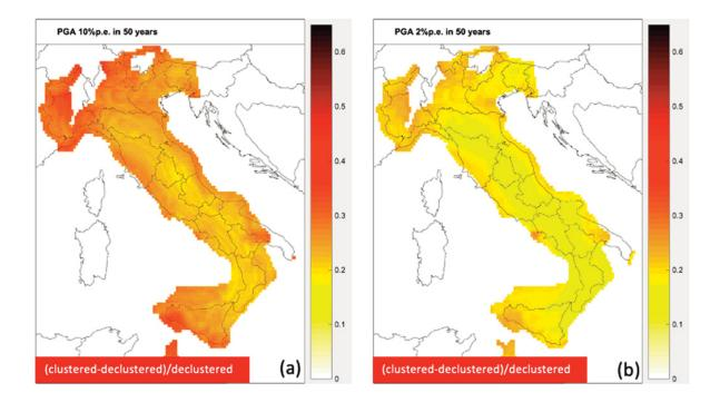
**Figure 11.** Variations of the (a) 10% PoE in 50 years, and (b) 2% PoE in 50 years PGA when the effect of clustered earthquakes are included to the maps of Figure 7b and 7c, respectively, according to the procedure described by Marzocchi and Taroni [2014]. The maps show only the sites with a PGA above the 25<sup>th</sup> percentile.
