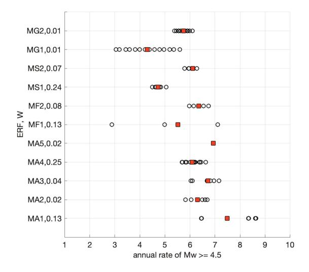
Figure 4. Distribution of rates of occurrence for earthquakes with  $M_w$  larger or equal than 4.5, as evaluated by the 11 ERMs and their sub-models (open circle). Red squares are the mean rate of each ERM. The y axis reports the ERMs with their own code and final weight (see Section 6).
