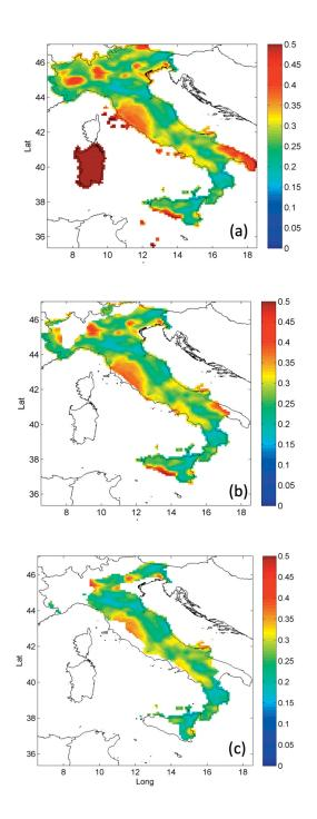
Figure 8. CoV (equation 2) map for the 10% PoE in 50 years PGA (Figure 7b). (a) CoV for the whole territory; (b) CoV for the sites of Figure 7b with PGA above the 25<sup>th</sup> percentile; (c) CoV for the sites of Figure 7b with PGA above the 50<sup>th</sup> percentile.
