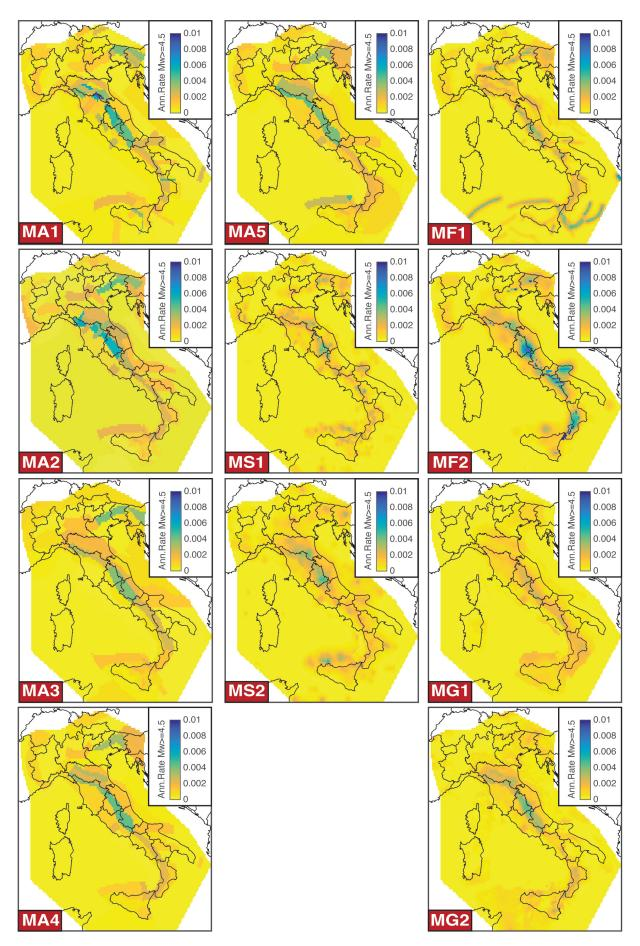
Figure 3. Mean annual earthquake rates for  $M_{\rm w} \geq 4.5$  of each ERM.
