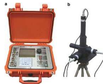
a) RMT receiver device, b) Magnetic coils
