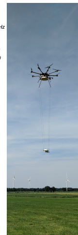
We used the MagArrow OPM suspended below the MGT-Arealis octocopter and flew a semi-airborne EM test survey near Merfeld, Germany (cf. Figure 1).
