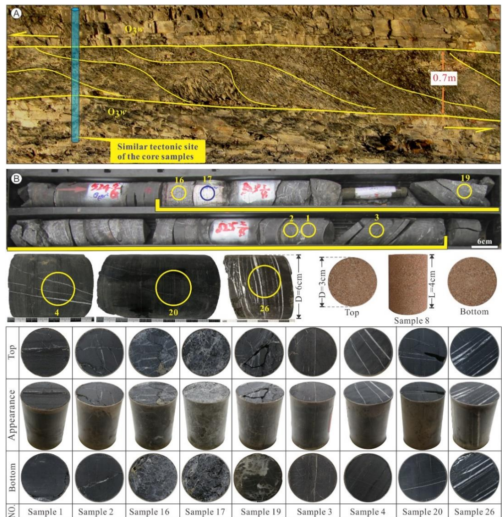
Figure 1. (A) Outcrop of a regional fault in shale strata in Chongqing municipality constituting a similar tectonic site to that of the core samples from well HD-1 used in this study; (B) images of well HD-1 cores and the 10 (i.e., 9 shale and 1 sandstone) samples used for permeability testing.
