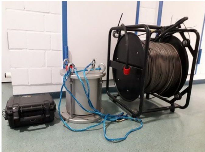
Figure 3: “Mobile Ocean Bottom Seismometer” (MOBSI) system: cable drum (right), broad band seismic sensor & data logger (middle) and control unit/computer (left). Modified from Ryberg et al., 2018.
