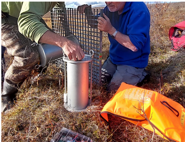
Figure 3: Shallow water ocean bottom seismometer. The cylinder containing the recorder and sensor is mounted on a metal grid.
