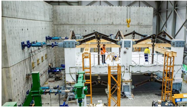
Figure 10: Global view of the building structure sub-assembly tested and building model geometry.
