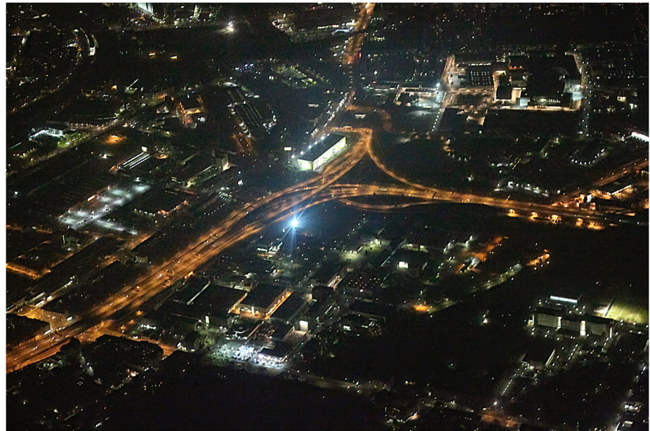
Figure 1. Aerial photo taken over Berlin on 15 March 2012. The dynamic range of night scenes is extremely large, ranging from diffuse reflection of starlight and skylow from unlit surfaces (which appear black here due to underexposure), to direct views of the radiant elements of luminaires (e.g., the overexposed bright point).
