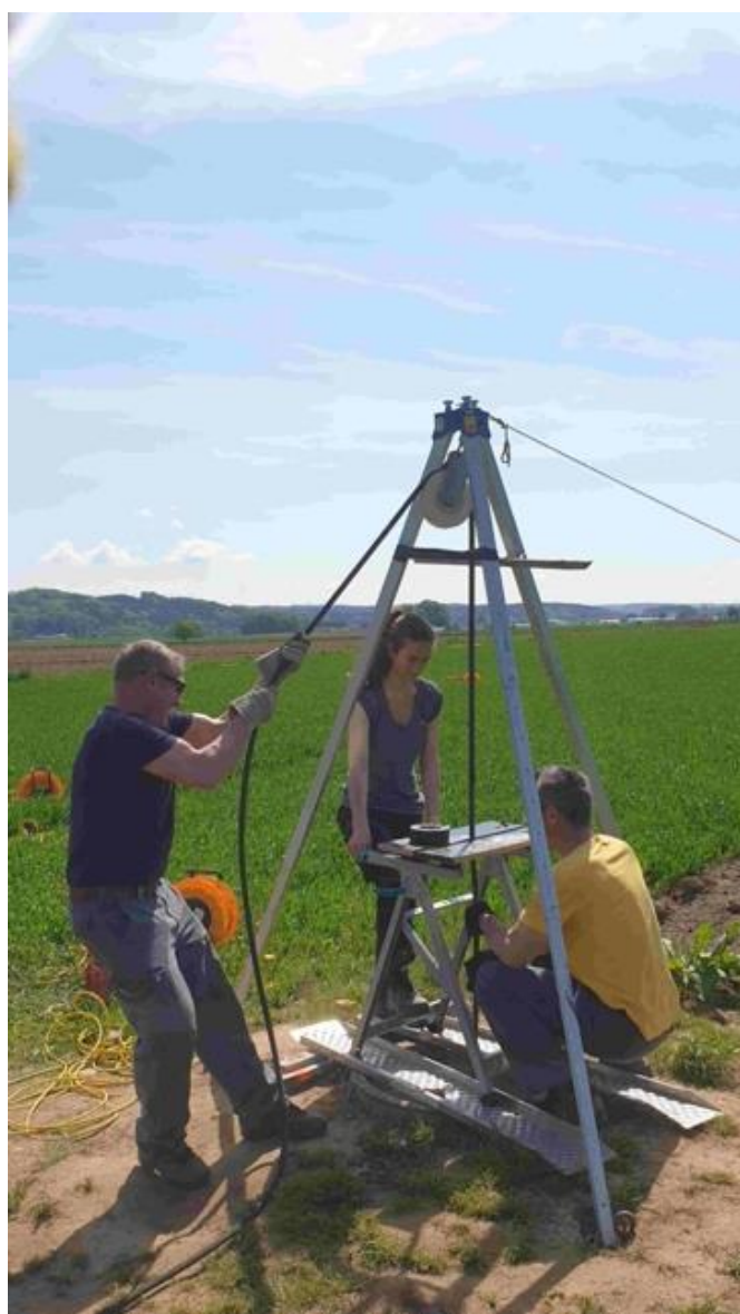
Figure 1: We orient the SH-source manually using the torsionally stiff hose and secure it at its position by clamping the hose between the two boards of a workbench.
