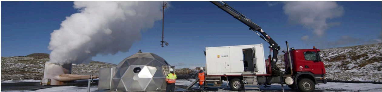
Figure 2: The methodology of well sampling of high-temperature geothermal wells using well logging slick-line equipment and a lubricator pipe.
